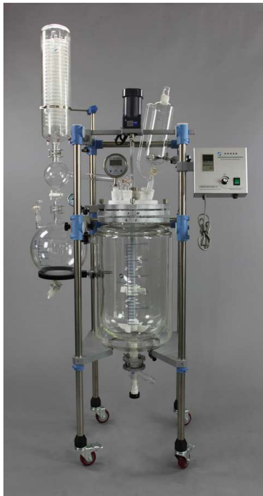
Distillation Separation Receiving For both separation and distillation receiving. No need to stop reaction or release vacuum when discharging condensate. Easy valve control can help on continuous receiving.
